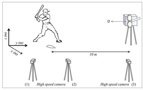
Figure 3. Setup for the oncoming ball hit
