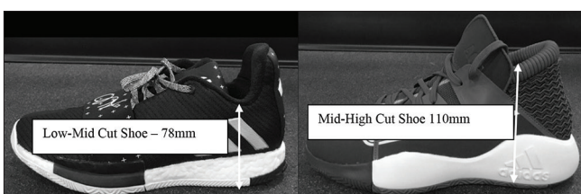
Figure 2. Collar height differences of Adidas™ Harden Vol 3. Low-Cut and Adidas™ Captain Marvel basketball shoe
