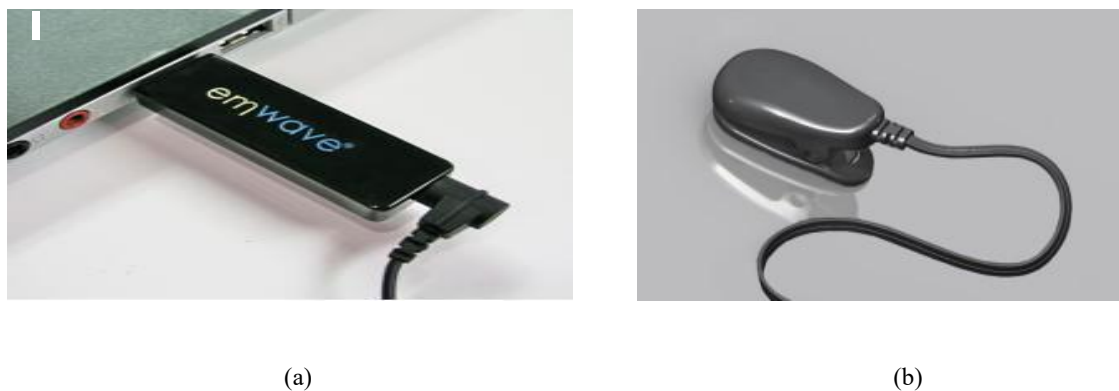
Figure 1. (a) emWave's USB key with the pulse sensor plugged in (b) Photoplethysmograph Ear Sensor
