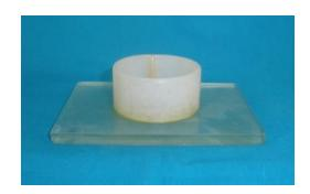
Figure 1: PVC cylinders were fixed on glass slabs by sticky waxed on glass slabs by sticky wax
